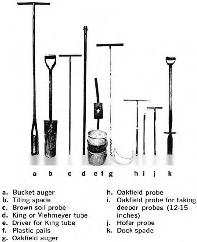
FIGURE 11.2 Hand tools for soil testing.
